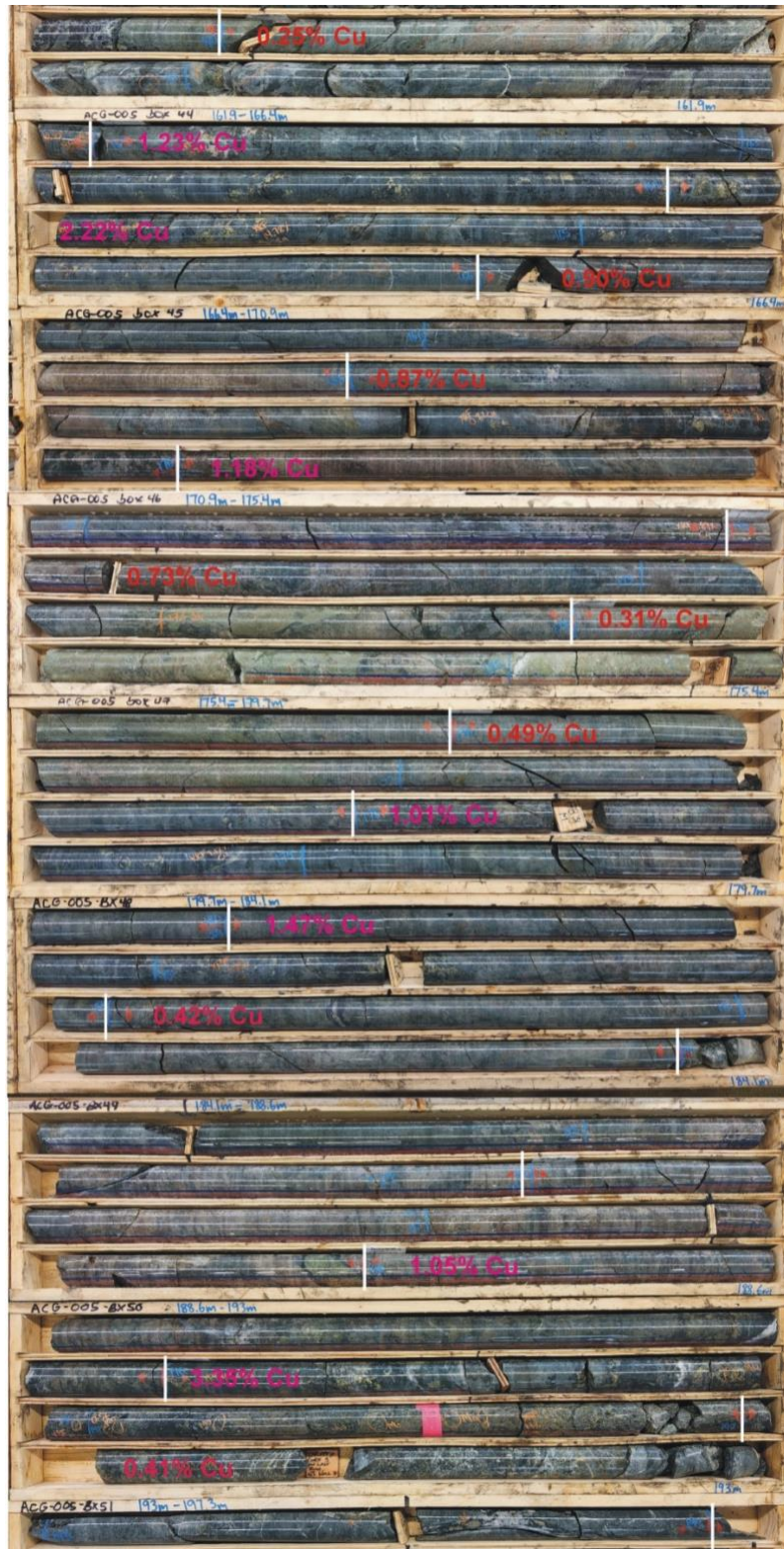
Figure 4– Hole ACG-005: Section of High-Grade Skarn Mineralization, 30m @ 1.03% Cu and 0.33g/t Au from 162m showing garnet-diopside (silicate) skarn with interstitial ragged blebs of chalcopyrite up to 10cm in size.
