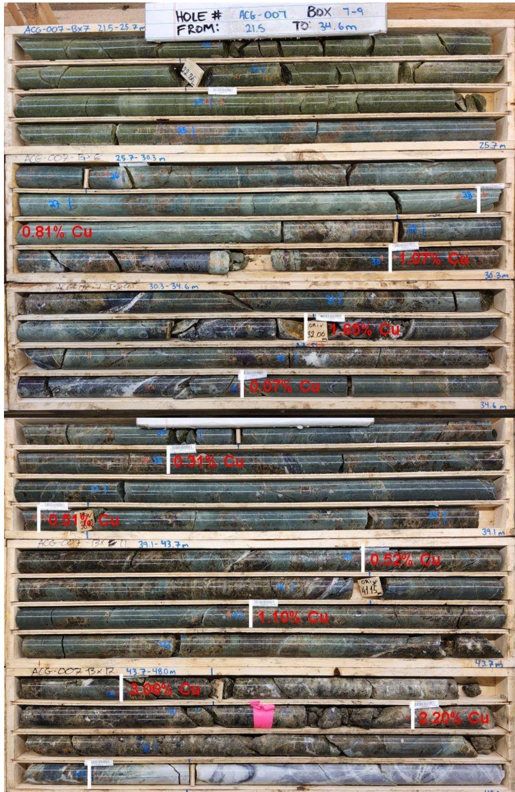
Figure 6 – Hole ACG-007: Section of Copper Skarn Mineralization, 19m @ 1.05% Cu from 28m within 43m @ 0.65% Cu from 16m showing garnet-diopside (silicate) skarn with interstitial ragged blebs of bornite up to 5cm in size.
